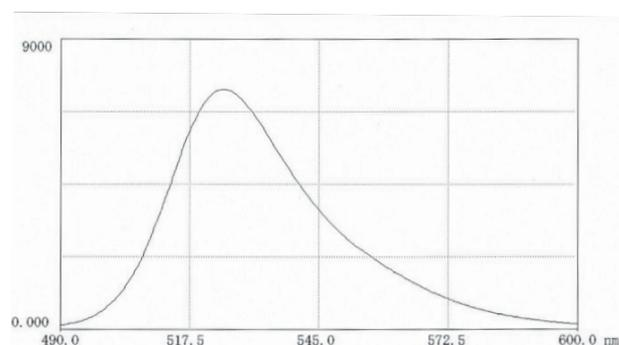
Fig. 2 Fluorescence scan of FITC-Polysucrose 70 in 0.025M borate pH 9.0 (9.9 mg in 50 ml buffer) Excitation 493nm; Emission 523nm
